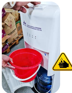
再按熱水掣將熱水全部排出 Press the hot water button to release all hot water
